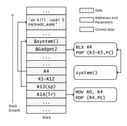
Fig. 6: Stack layout after loading the payload.
